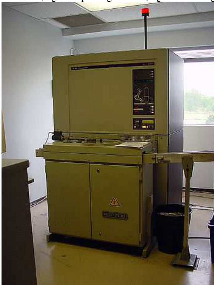
A Philips PW1606 X-ray fluorescence spectrometer with automated sample feed in a cement plant quality control laboratory
